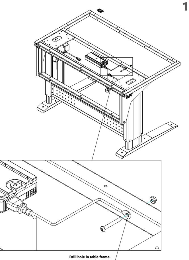
Attach grounding cable with screw + nut.
