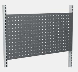
3-521-36 **Perforated tool panel 900 mm.**Hole dimension 9x9 mm and hole distance c/c 38 mm. Also available in 670 mm.
