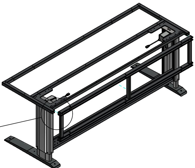
Slide the rear frame with the screws in to the slots of the top frame.
