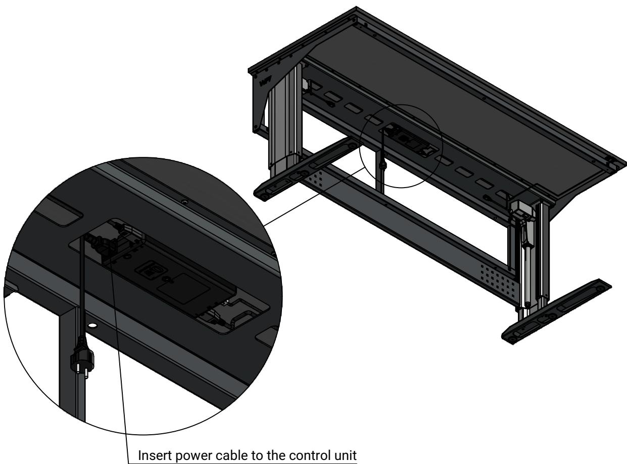
Insert power cable to the control unit
