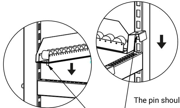
The pin should be in any hole in the pipe depending on which plastic back you use
